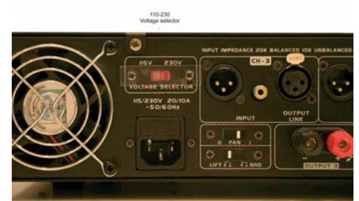
110-230 Voltage selector Fuse Dual fan speed, setting 0 = silent mode, setting 1 = full fan speed Ground IRT
